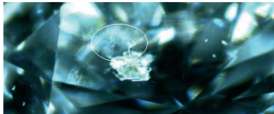
Laser drilled with burn on entry facet
